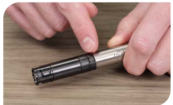
Replace the ISE module every 6 months, or as needed.
